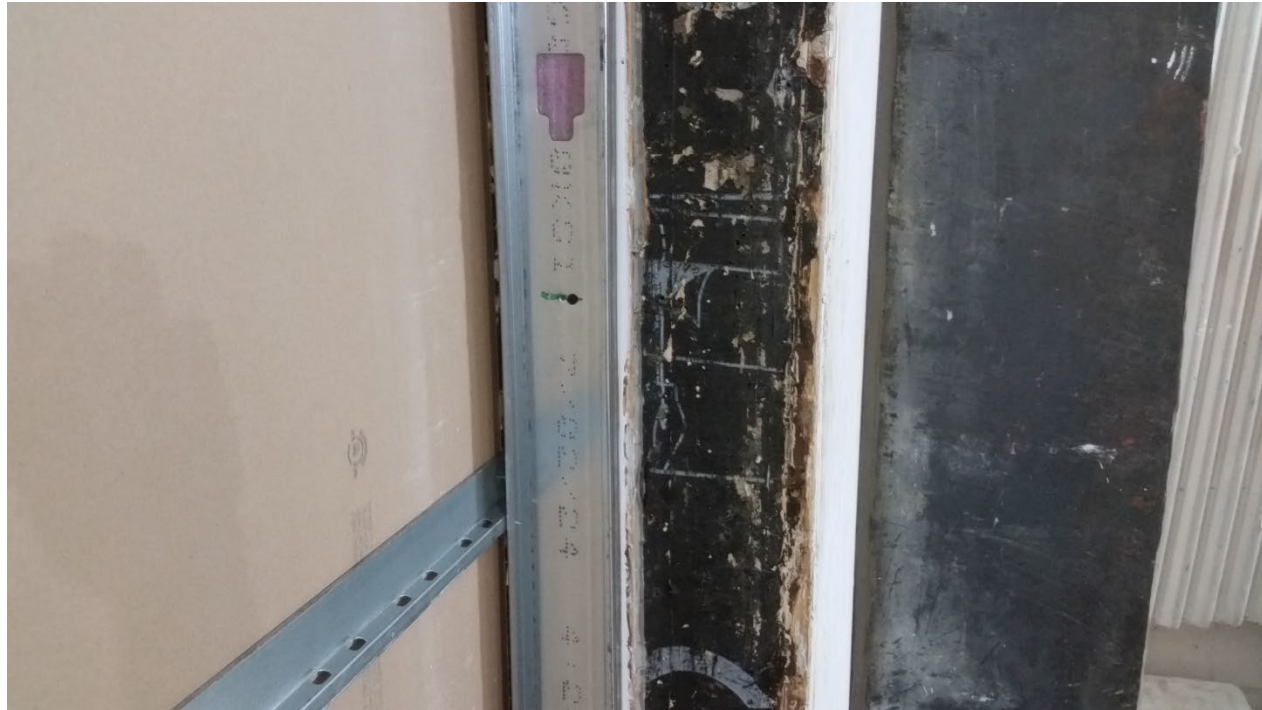
Figure 5 – Detail of side stud fastened to test frame, viewed from receive room side
